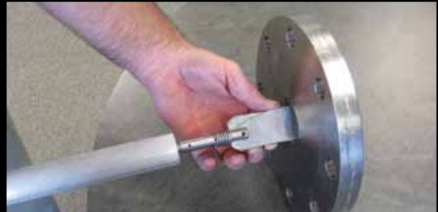
The paddle automatically springs open after it is through the wall.
