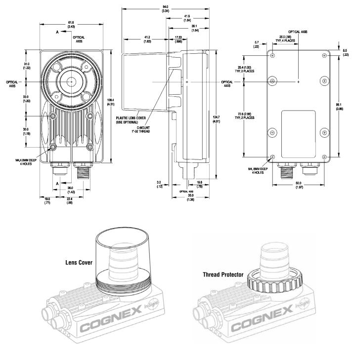
The lens cover included with In-Sight 5000 Series vision sensors provides wash-down and dust protection. A thread protector, also included, protects the threads when the lens cover is not used.
