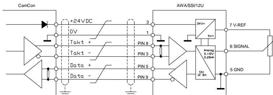
**Attention:** At the CamCon an SSI-singleturn encoder with 4096 steps, Gray has to be chosen as the measuring system at this AWA/SSI version 2.
