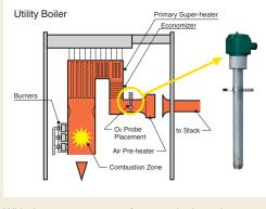
With the measurement of oxygen in the exhaust gas the flow of fuel can be controlled for optimum burner efficiency and minimum environmental effects.
